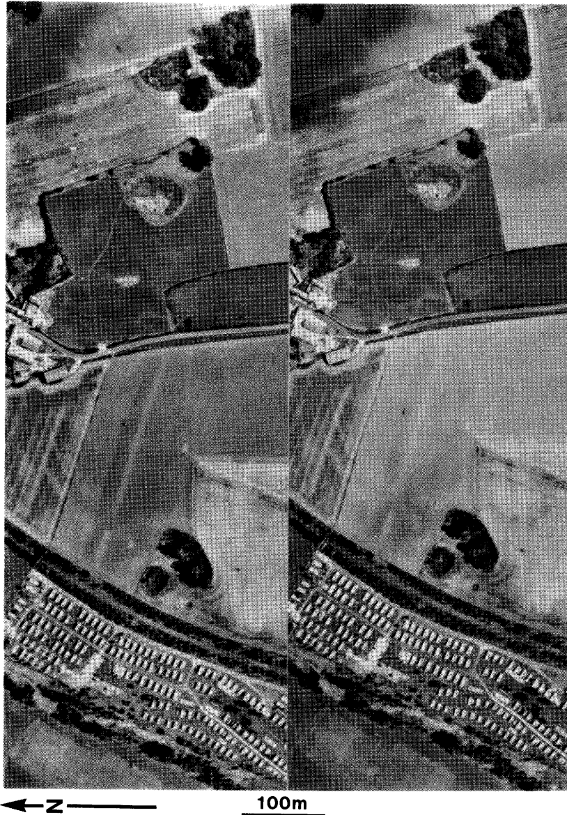
FIG. 8. Stereo pair of photographs of subsidence hollows near Hutton Conyers (see Fig. 10 for location). Note also the bluff and alluvial flat just below the caravan park at the bottom of the photographs. To view this use a pocket stereoscope or hold a 15 cm high piece of grey card vertically between the two photographs in line with your nose, stare at the photographs, but let your eyes relax. You should see three images with the central one in 3D.
