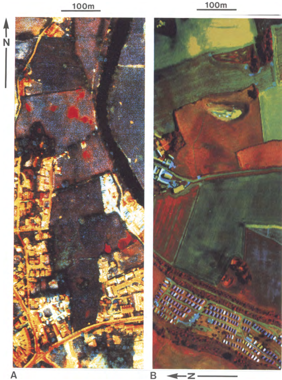
FIG. 6. (A) Multispectral scanner image of subsidence hollows in the area south of Low Common Farm and north of Ripon Clock Tower (see Fig. 10 for location and Fig. 7A for explanation). This image was gathered under complete cloud cover. It uses bands 11, 9, 10 and is scaled giving a false colour image that shows water filled hollows as red on a purple-green background. This band combination also shows vegetation changes in subdued subsidence areas. This image has slight oblique distortion (Fig. 10). (B) Multispectral scanner image of subsidence hollows near Hutton Conyers (see Fig. 10 for location and Fig. 7B for explanation). This image uses bands 7, 11, 5. It was gathered in full sunlight and has been scaled. The false colour image shows variations in soil and vegetation. Compare with Fig. 8 of the same area.
